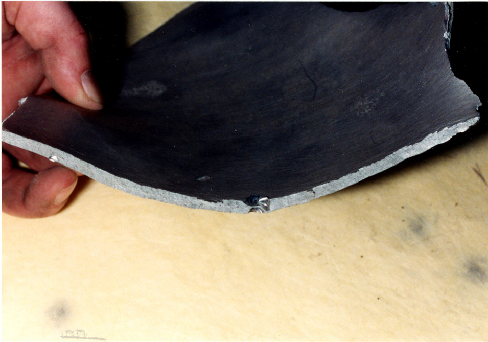
49. Close-up view of the edge of the aluminum tank fragment
